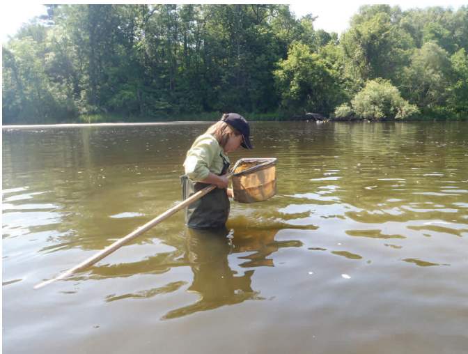
Using a “D” net to collect benthic invertebrates
