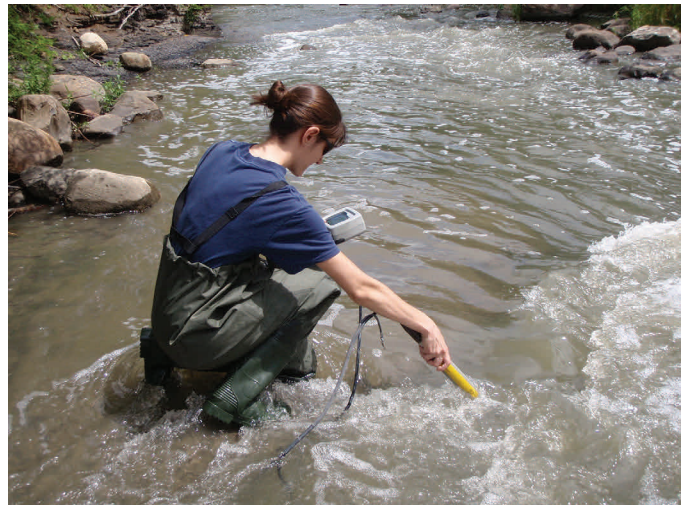
A staff member using a YSI to collect water quality data
